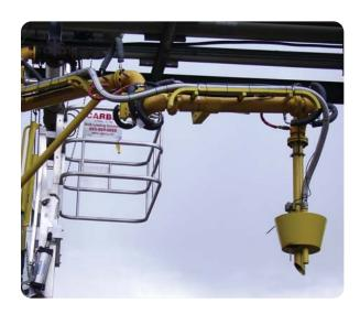
Some loading arms can even be heated. This comes in handy if there are hot products that tend to crystallize or solidify while inside the arm. Heating is done using either electric tracing or liquid tracing.<sup>5</sup>
