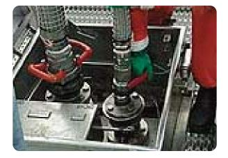
There are times when hoses are the best solution for the job. Certain chemicals such as hydrochloric acid and bleach require hoses that are specially lined to avoid corrosion. Hoses are more flexible than loading arms but they are also more likely to wear out. Hoses are heavy, bulky and create a fall hazard. They're a constant cost because they have to be replaced often.
