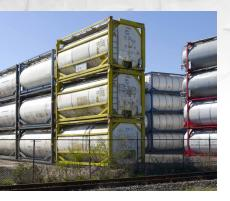
The chemical industry, the food industry and a variety of others make use of ISO containers, also known as isotainers and seatainers. These are essentially round tanks fixed in rectangular frames to allow for easy stacking on ships. When they're not being transported via ship or barge, these containers are transferred onto different types of flatbed trucks and driven to their final destinations.
